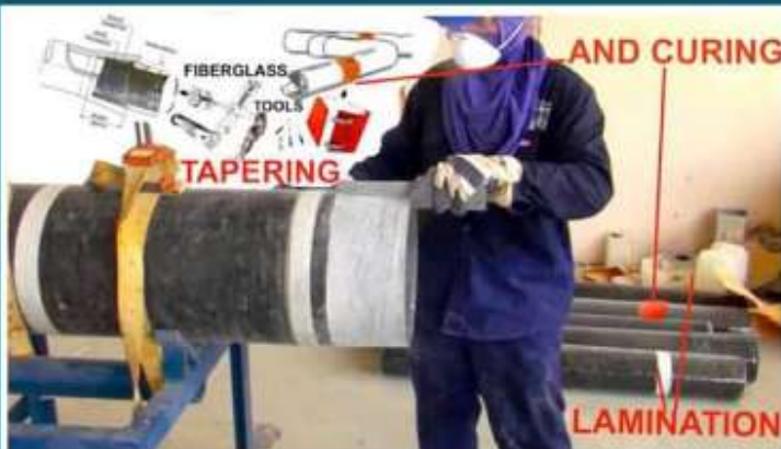
TYPICAL CONSTRUCTION OF FILAMENT WOUND RTR PIPE
